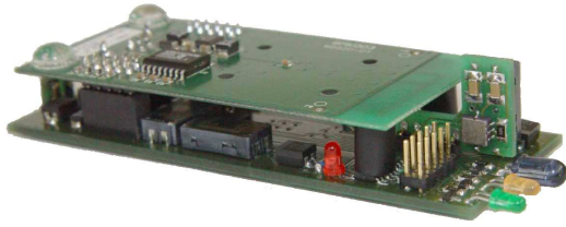
Figure 1: First prototype board of the BlueWand with orthogonal sensor fin and Ericsson Bluetooth module on top.
